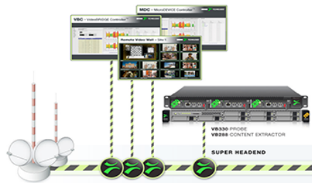
Figure - VB288 is typically deployed in the master head-end prior to encryption.
