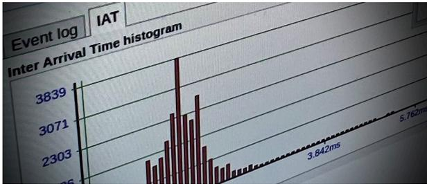
received is over time. It shows an accumulated count of the number of IAT measurements that fall within each presented bin interval. Vertical green lines indicate the maximum and minimum IAT values observed. The user can customize the scales.
