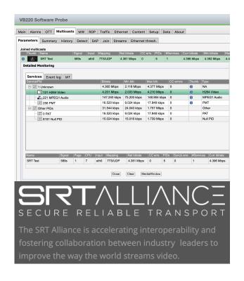
for further analysis. This includes MediaWindow visualisation, TR 101 290 analysis, content capture and thumbnail mosaic. Key parameters such as round-time and lost-packets are displayed. The VB120 can also send out any two media streams currently being monitored by the probe as an SRT-formatted stream. This capability is typically used for ad-hoc transport of content across an IP network for remote live viewing or recording. SRT support is a standard feature on the VB120.
