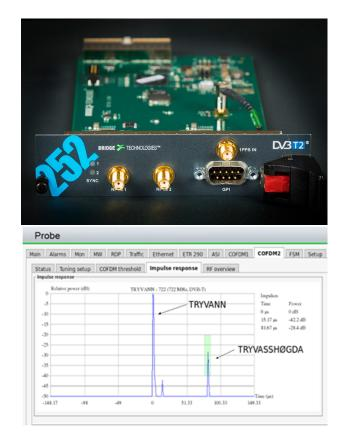
reflection changes in time or power. Impulse response analysis results are presented as a user-friendly graphical GUI, facilitating reflection measurement interpretation.
