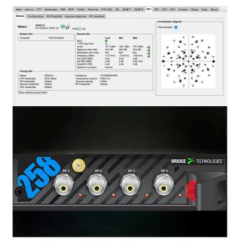
conversion of any received RF stream into an IP/UDP stream, which is then made available via the SRT standard. SRT (Short Reliable Transport) allows for reliable UDP streaming across Internet-type media, and through this it is possible to gain central access to streams that would otherwise be hard to access.
