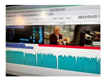
initiated either manually, by a preset time schedule or by trigger events such as any of the probe alarms or even SCTE35 ad-insert events. For the event triggered recordings a pre-fill buffer is also stored, ensuring the trigger cause itself is captured to the same recording. The concurrent record option comes in steps of 100 up to a total of 200.
