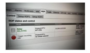
available centrally signals that are normally only available locally. RDP<sup>TM</sup> also facilitates a simpler descrambling process for scrambled signals, by transporting the stream to the NOC, head-end or anywhere else for visual monitoring.
