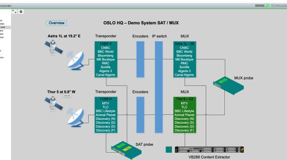
charts, network diagrams or geographical map locations. The graphics view systems diagrams can be configured to be shown in a carousel manner to the operator to cycle through as much relevant information as possible. Each graphics diagram is recursive in nature, where the user can click on an object in one drawing and drill into another. Links can be made to tunnel straight into monitoring probes from the top-level graphical view.
