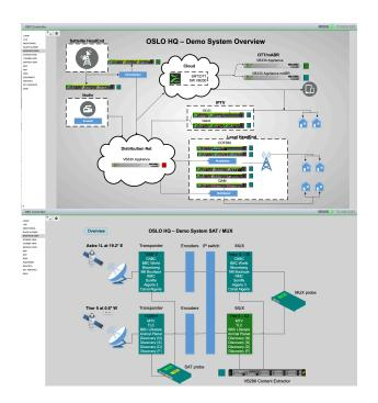
physical rack layout diagrams, logical signal flow charts, network diagrams or geographical map locations. The graphics view systems diagrams can be configured to be shown in a carousel manner to the operator to cycle through as much relevant information as possible. Each graphics diagram is recursive in nature, where the user can click on an object in one drawing and drill into another. Links can be made to tunnel straight into monitoring probes from the top-level graphical view.
